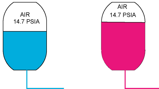
Figure 2: A closed tank with no bladder has free space when the hydronic hot water system is cold. As the temperature within the system rises, the water expands into the free space within the tank.
